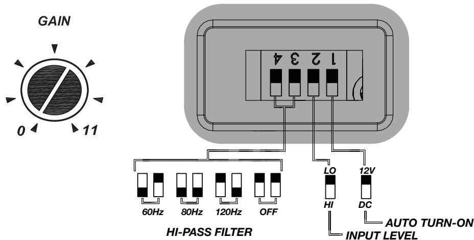
**Automatic Turn-On Selection:** The PXA series offers two automatic turn-on modes that can be selected on the end panel; +12V or DC Offset. Using the DC Offset mode causes the REM terminal wire to have +12V out for turning on additional amplifiers.
