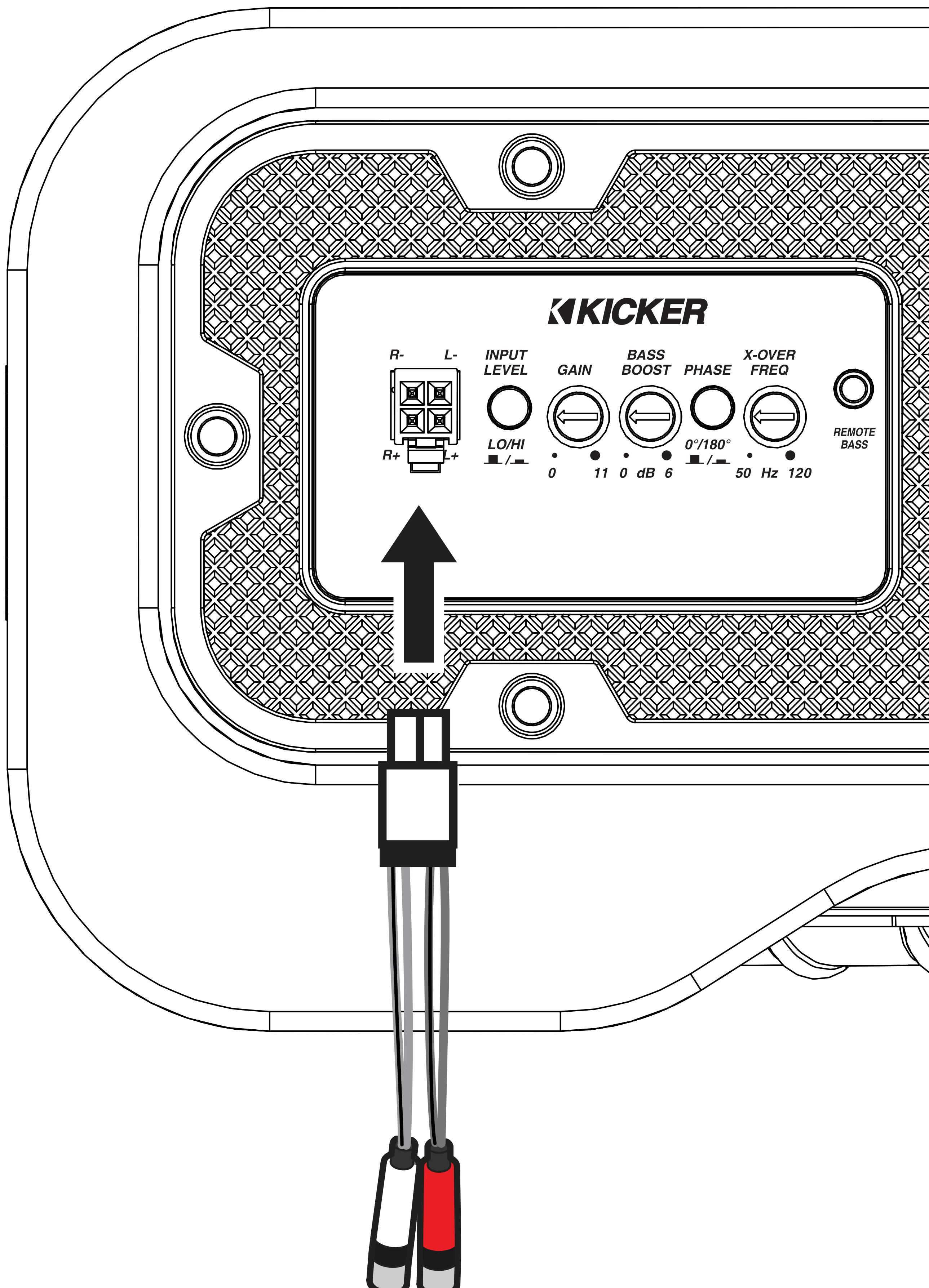
If needed, cut off the RCA connections to use hi-level input, or use the [KICKER KISL Speaker-RCA Converter](#).
