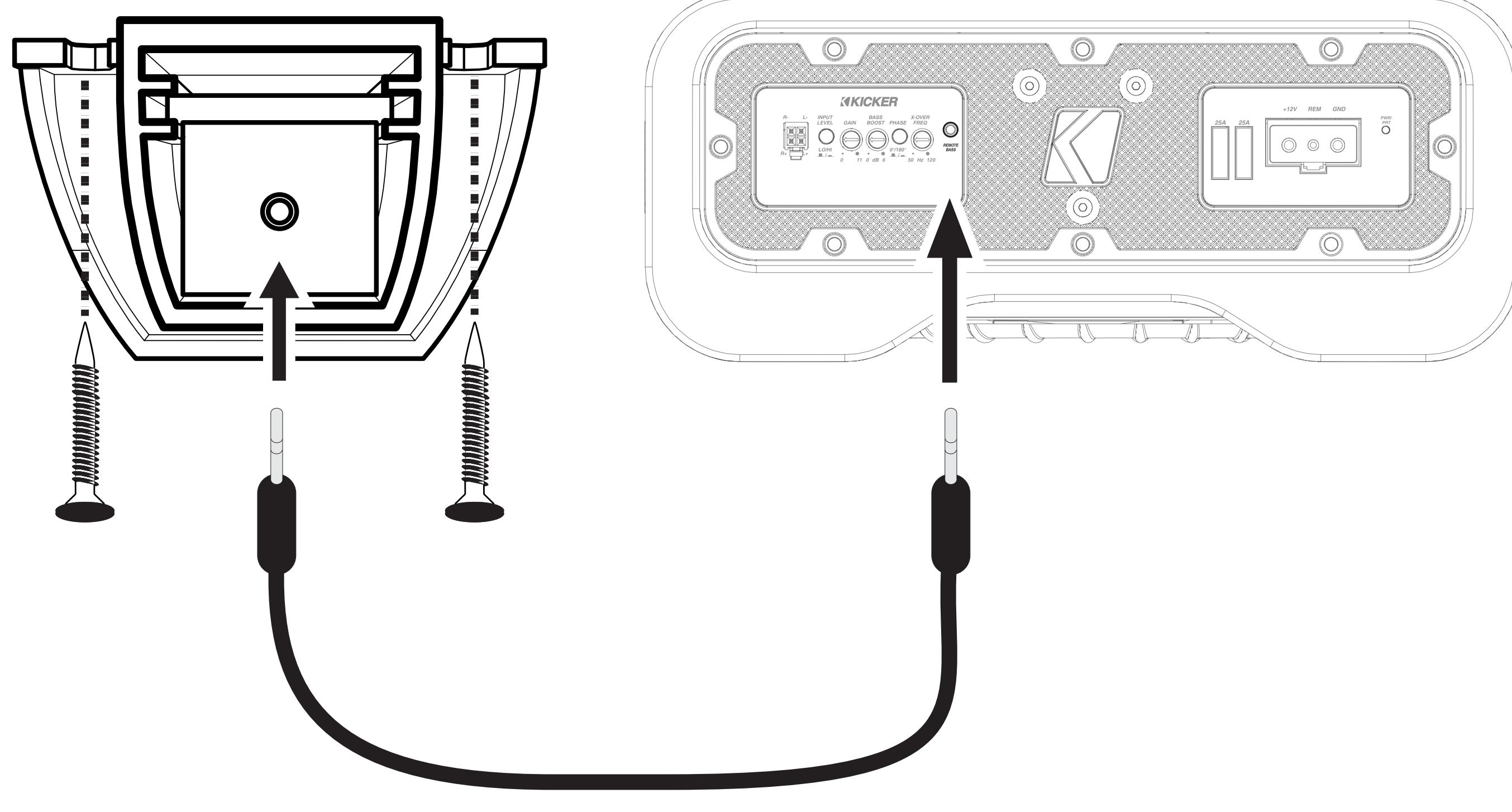
Connect the cable to the remote and the Remote Bass connection on the amplifier
