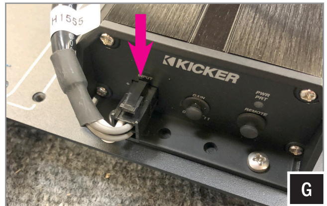
G. On the 500.1 amp, compress the locking tabs and pull the connectors to disconnect harnesses from the amplifier.
