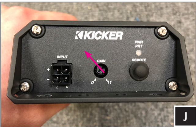
J. Remove gain control plug, starting from zero adjust gain control clock wise to the position shown. Once tuned re-insert plugs and switch cover.
