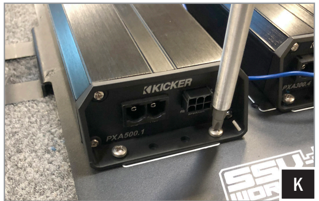
K. Transfer the 500.1 amp to the Ride Command compatible amp tray. Fasten the amp to the tray with your existing M4 hardware. We recommend applying Threadlocker.
