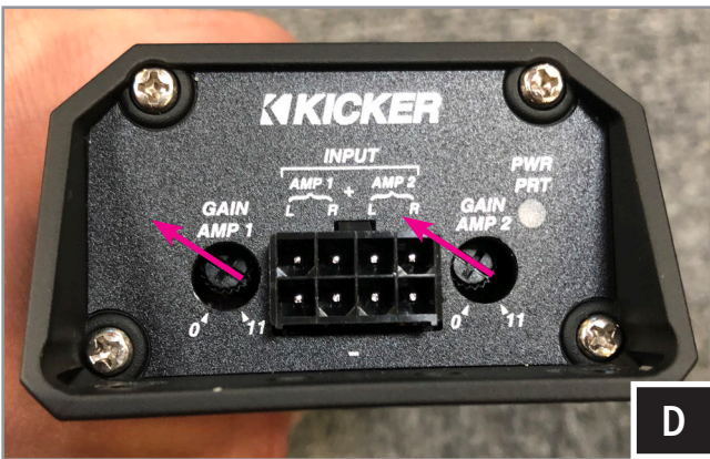
D. Remove gain control plugs, starting from zero adjust gain control clock wise to the position shown. Once tuned re-insert plugs and switch cover.
