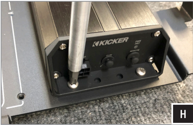
H. With the amplifier disconnected, unscrew the (4) screws that secure the amp to the amp tray.
