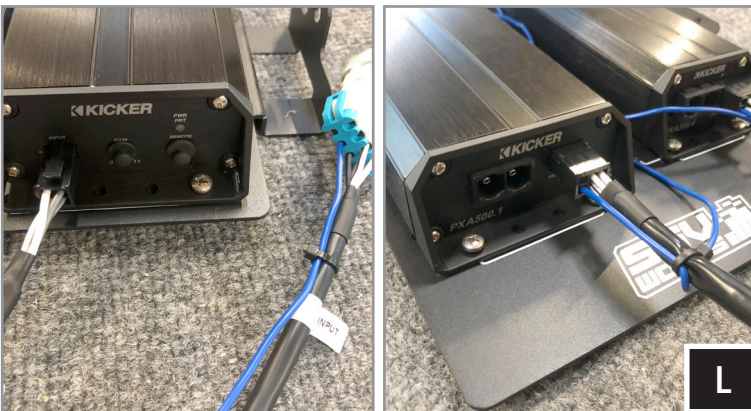
L. Connect harness B-H1811 to 500.1. The 4-pin connector to the input side of the amp and 6-pin connector to the output side of the amp.
