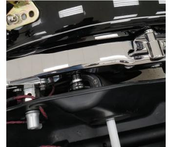
8. Drill a 3/4" hole in each bag as pictured and install the supplied rubber gromets.
