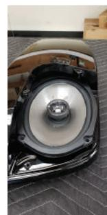
4. Place the bracket on the back side of the speaker. Install a bolt through the bracket and speaker from the back side, then position the speaker nut on top and tighten. Using the factory screw, attach the outside of the bracket to the lid.
