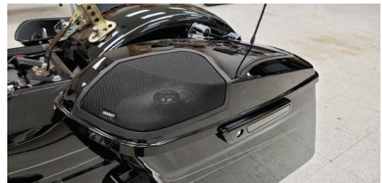
*Note:* If not already flashed for rear speakers, it will now be necessary to flash the motorcycle for 4-speaker set up using the KICKER flash programmer of the Techno Research Centurion. Follow instructions for Flash Programmer to complete this task.
