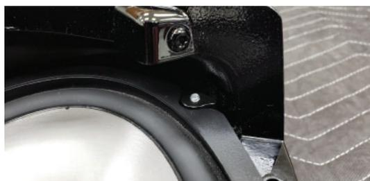
5. install the factory latch lever using the factory screw and supplied rubber grommet.
