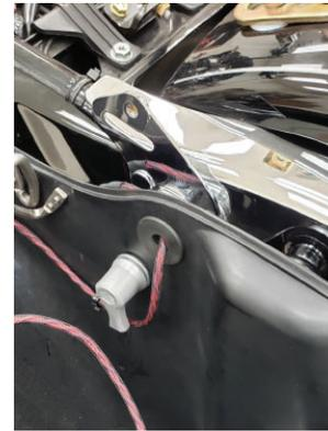
9. Using the included zip tie mounts and zip ties, route each wire as show in the picture to secure the bag harness.
