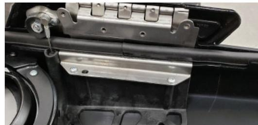
2. Install the factory latch and hinge assembly to your new KICKER lids using the factory screws.
