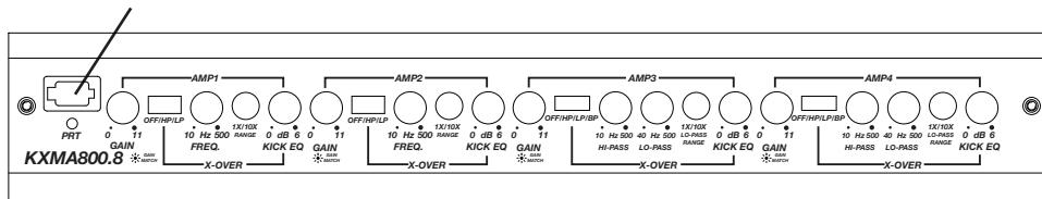
**Automatic Turn-On Selection:** The KXMA series offers three different automatic turn-on modes that can be selected on the end panel; +12V, DC Offset, and Audio. Using either the DC Offset or Audio mode causes the REM terminal to have +12V out for turning on additional amplifiers.
