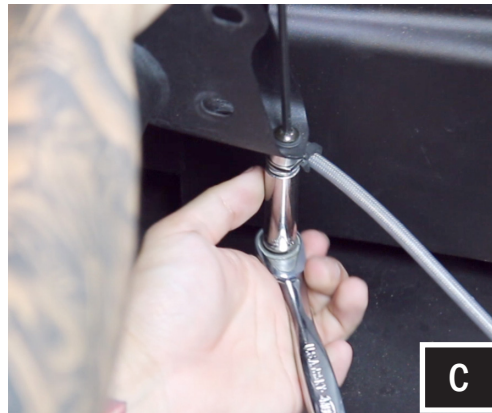
C. Remove the factory 10mm nut and bolt from the brake line. Place the washer on top of the factory bracket and push the long M6x25mm screw through the top. Then attach the brake line, spacer, washer and nut. Then hand tighten.
