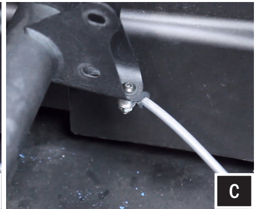
C. Remove the factory 10mm nut and bolt from the brake line. Place the washer on top of the factory bracket and push the long M6x25mm screw through the top. Then attach the brake line, spacer, washer and nut. Then hand tighten.
