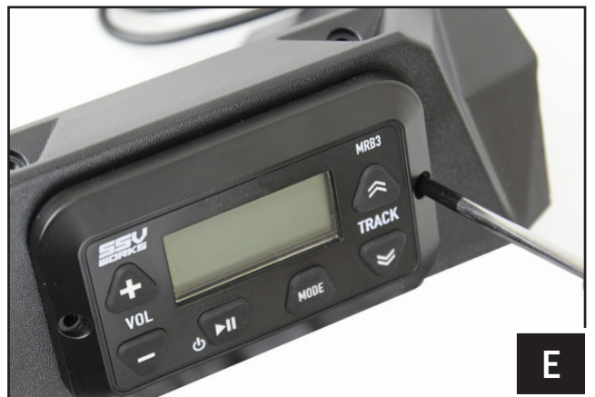
E. Fasten the MRB3 Remote to the dash kit using (2) M3 screws.
