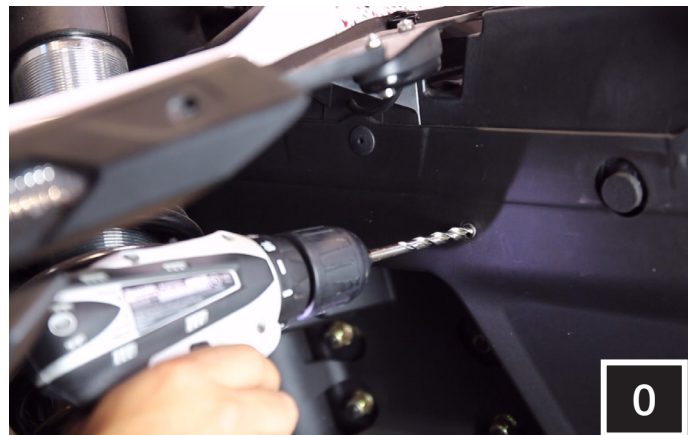
O. Drill a larger hole through the pilot hole using a 1/4" drill bit. Be sure to move the amp plate out of the way before drilling.
