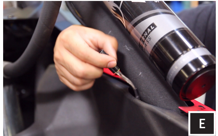
E. Route the rear speaker harness (B-H1150) along the factory wires in the engine compartment and pull up through the small space between the bed panel and cage tubing on both passenger and driver sides.
