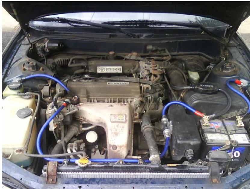
The wire on the left is the ground from the chassis to the engine block. The center wire is the charging wire and the wire on the far right is the ground from the battery to the chassis of the vehicle. The black jacketed wire coming off the left post (+) is the power wire that runs back the audio system.
