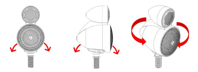
1. To adjust the rotation of the tweeter around the mid, remove the decorative plug at the back of the pod assembly. Using a 2.5mm allen wrench, loosen (do not remove) the bolt retaining the tweeter to the mid.
