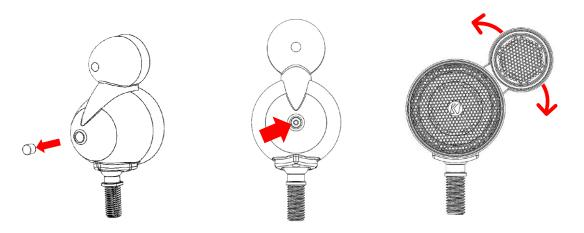
2. Rotate the tweeter to the desired location and retighten the bolt. Replace the decorative plug.
