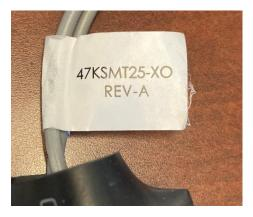
1. Connect the crossover terminals and receptacles to their respective mating connector on the KSMT25 pod assembly. The terminals on the 47KSMT25 crossover are all different sizes and types to prevent incorrect connection. Also, the crossover wire colors match the pod assembly wire colors.
