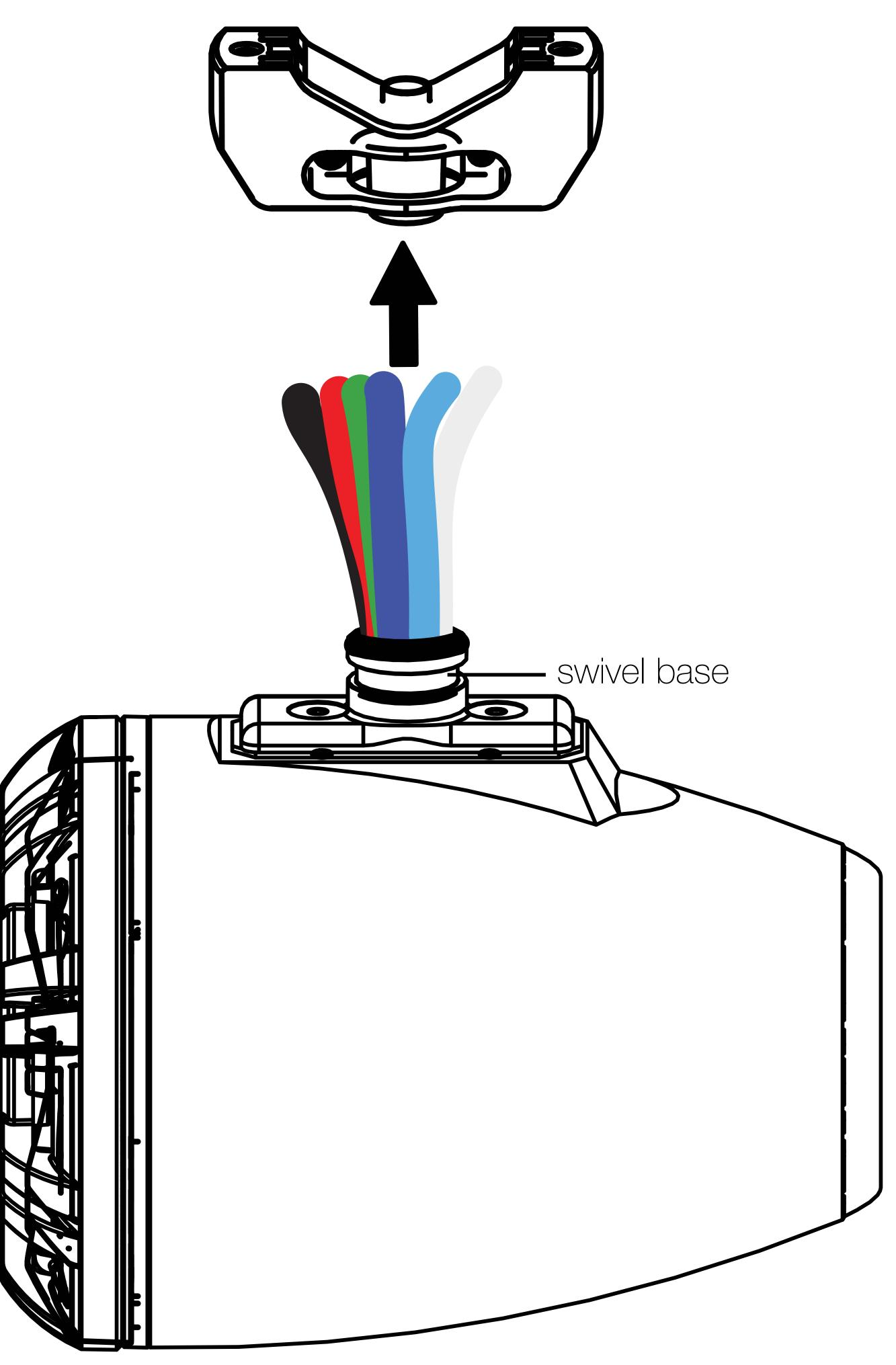
IMPORTANT: You must apply a thin layer of the included anti-seize compound to **ALL** threaded fasteners before installation.
