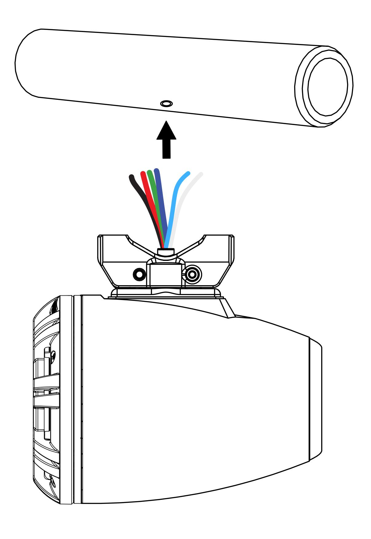
When hard-wiring the LED lighting, the black lead is +12V and the blue, red and green leads are ground.
