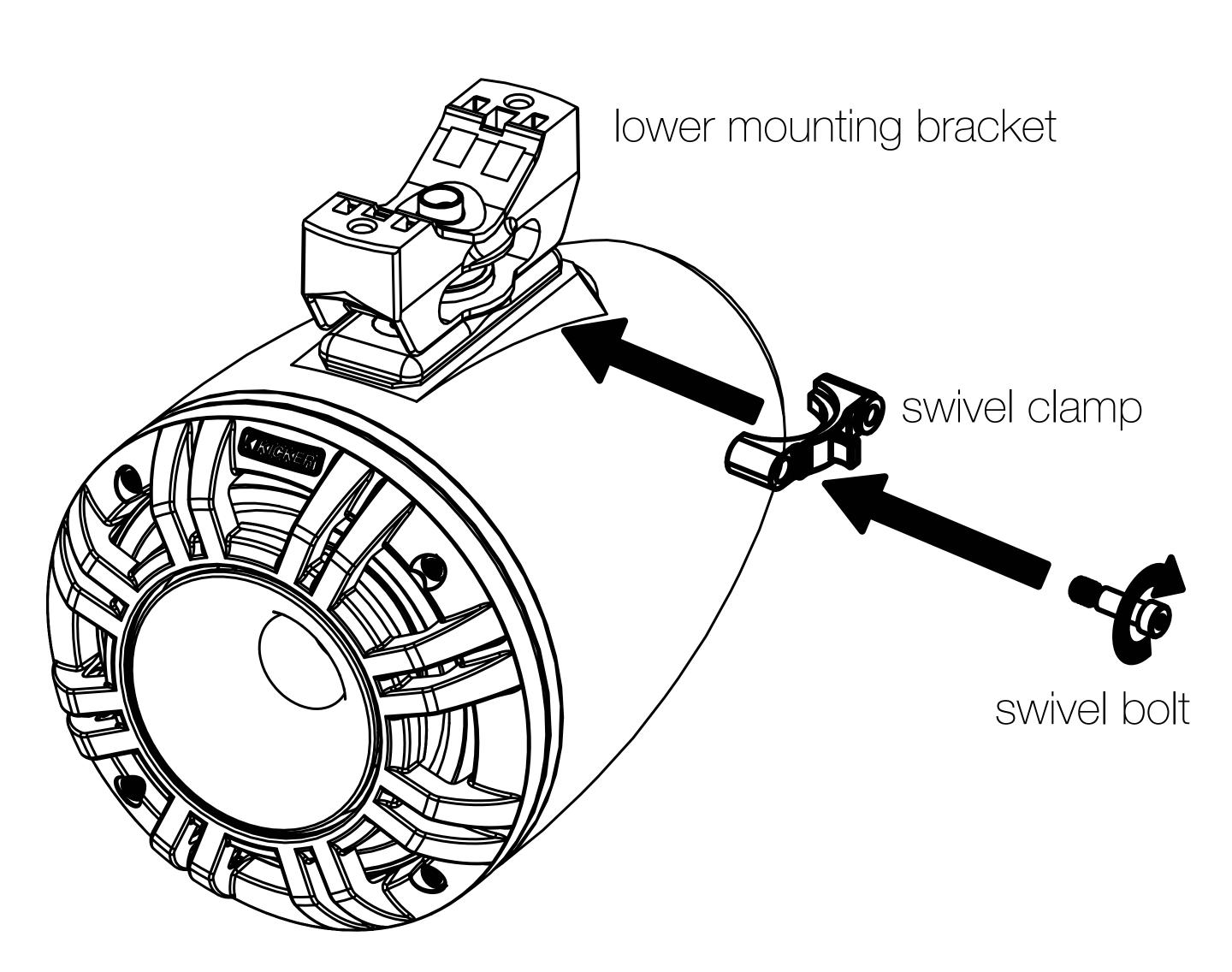
**Step 4:** Partially install the swivel lever, adjusting it to be loose (open) when the lever is parallel to the tube, then finish tightly securing the swivel lever to the enclosure using the included thumbscrew. When the swivel lever is locked in place, or closed, the bracket rotation assembly will be clamped tight.
