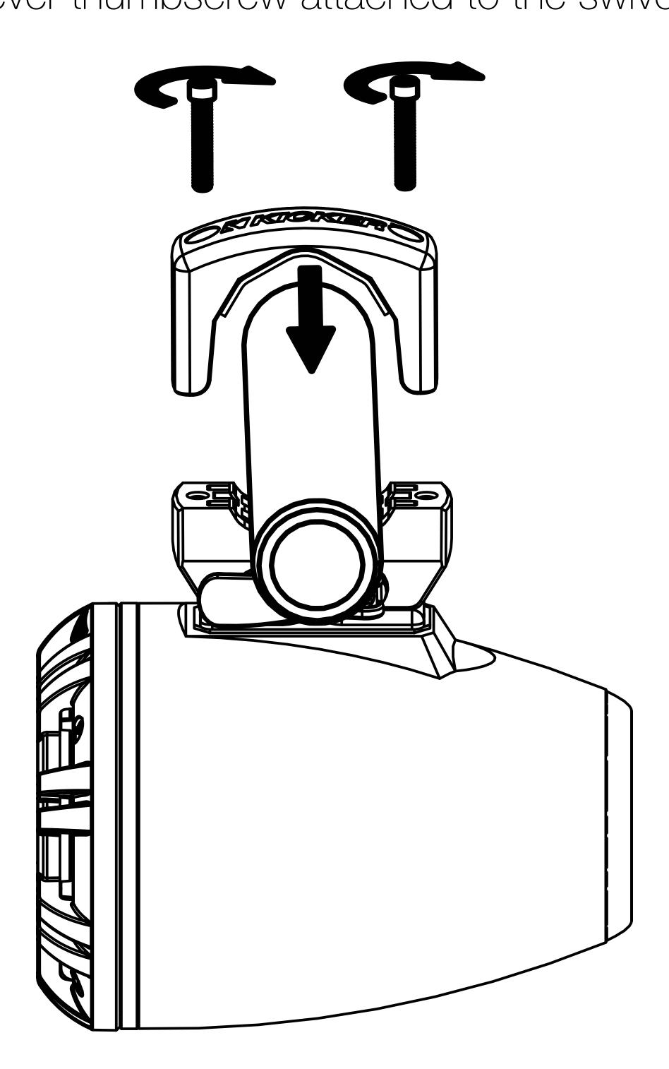
With the enclosure securely mounted, you may finish by opening the swivel lever and swiveling the assembly left or right. When you are satisfied with the orientation, close the swivel lever to lock the enclosure in place. If the enclosure is not locked tightly enough, tighten the thumbscrew.
