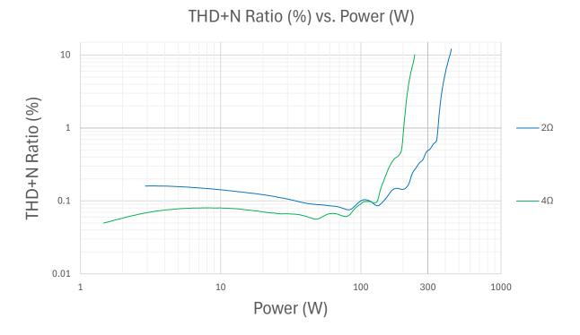
AMP1 and AMP2 - Power Bandwidth (4 $\Omega$ ) @14.4VDC
