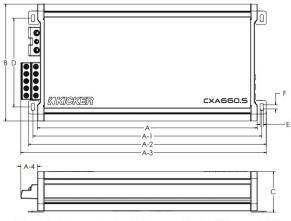
\* The use of vertical mounting brackets adds 2.1mm to total length and 4.5mm to total width
